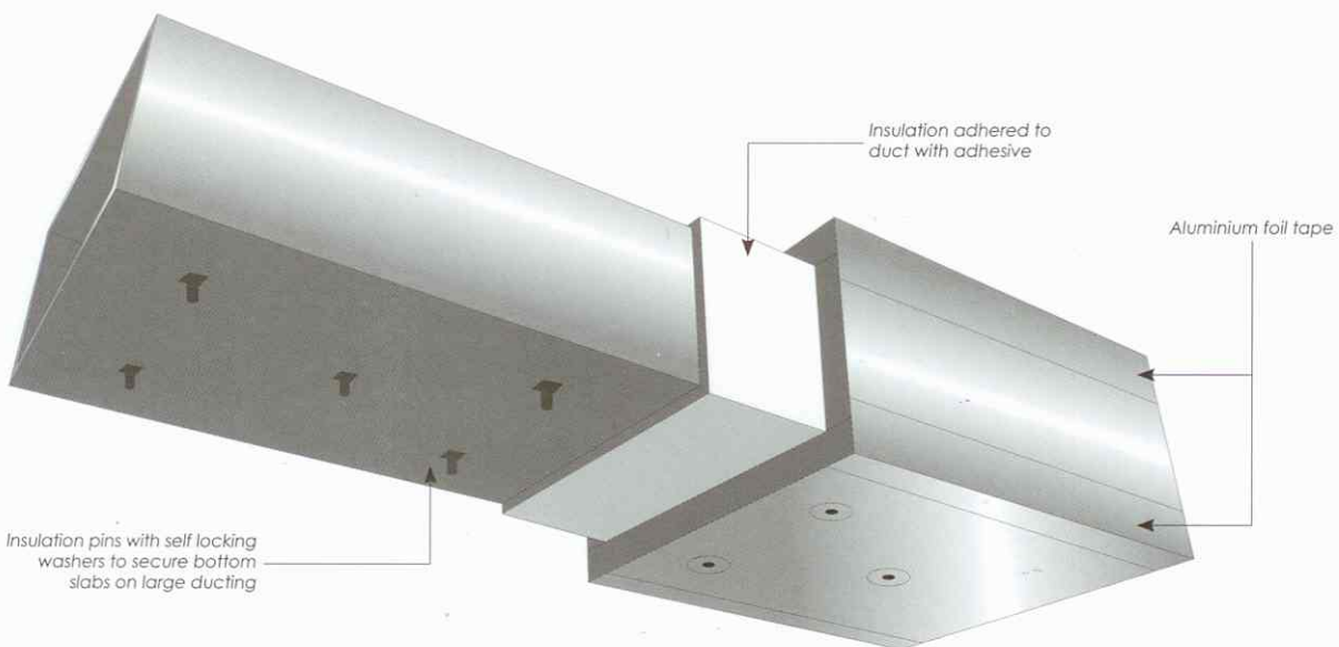
Fig.3 Installation of Evertherm Phenolic Foam Duct Insulation.
